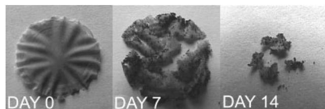
Figure 9 Biodegradation of chitin films in compost-soil mixtures (chitin film was completely degraded after 17 days).
